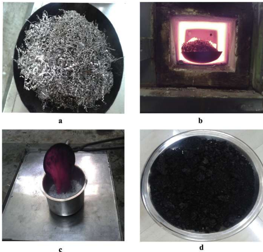
Fig. 2. Shodhana process of Teekshna lauha (iron turning). (a) Raw Teekshna lauha (iron turning), (b) red hot iron turning, (c) quenching process, (d) Teekshna lauha after shodhana.
