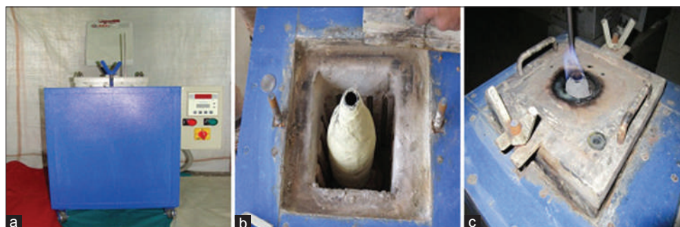
Figure 3: Rasasindura pictures: Preparation of RS in EMF. (a) EMF, (b) Placing Kupi , (c) Flame
