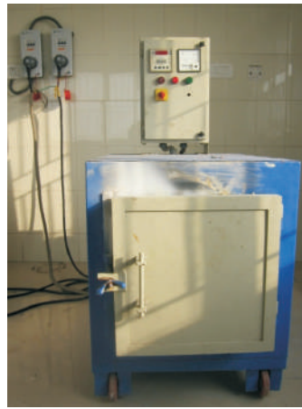
Figure 4 : Electric Muffle Furnace employed for incineration
