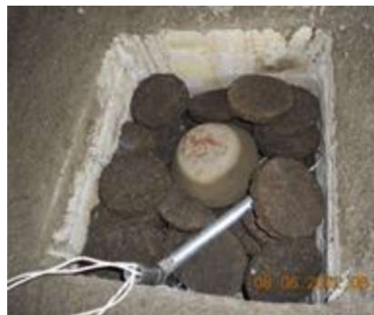
Fig. 1. Partly filled Varaha Puta with cow dung cakes
