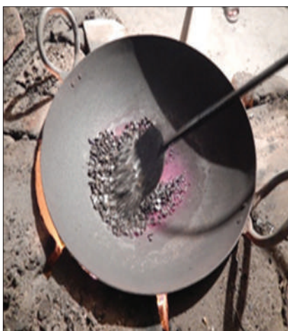
Figure 4: Roasting of Swarna Makshika in iron pan
